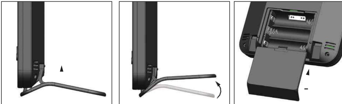
1. Remove the battery door of the main unit.
